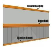
Skirting is usually around 6inches high around floors and normally made of same design and material as that of the floors. Primarily to protect walls daily from floor mopping and minor spillages on floors.
